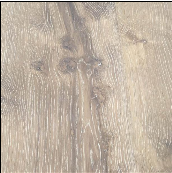
A knot cut at an angle to its long axis so that the exposed section is elongated.
